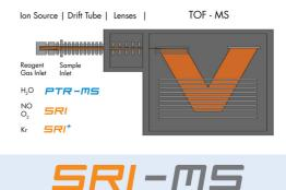
The IONICON PTR-TOF 1000 is also available with Selective Reagent Ionization - Mass Spectrometry (SRI/SRI<sup>+</sup>) featuring NO<sup>+</sup> and O<sub>2</sub><sup>+</sup> (SRI) or Kr<sup>+</sup> (SRI<sup>+</sup>) alternatively to H<sub>3</sub>O<sup>+</sup> as precursor ions created in the new ULTRA-PURE ion source (US Pat. 9,188,564).
